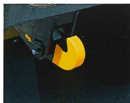
▲ Automatic tail gate locking device
