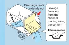
The discharge plate extends and stops past the back end of the body, making it easy to wash away any dirt remaining on the bottom of the body
