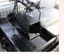
The body and tailgate are coated with an electro-deposition process to enhance rust prevention effects
