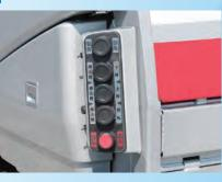
The loading switch control panel on the side of the loading hopper is angled to the rear left. This enables operation from side of the vehicle, and keeps the operator safe even with unpredictable movement of waste within the honner
