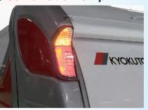
Specially designed LED rear combination lamps have been used as the tail lamps. These improve visibility both from behind and the side, making waste collection work even
